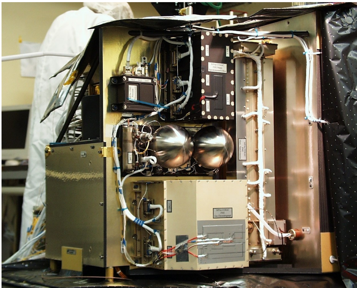
Fig. 84: A view of the COSAC experiment already mounted on the Lander. The hemispherical pressurised bottles in the centre contain the helium “carrier gas” required for the gas chromatograph. The gas chromatograph is mounted just below. The long device to its right is the housing of the Time of Flight mass spectrometer. Most of the electronics is housed in the black boxes above the pressurised bottles.
