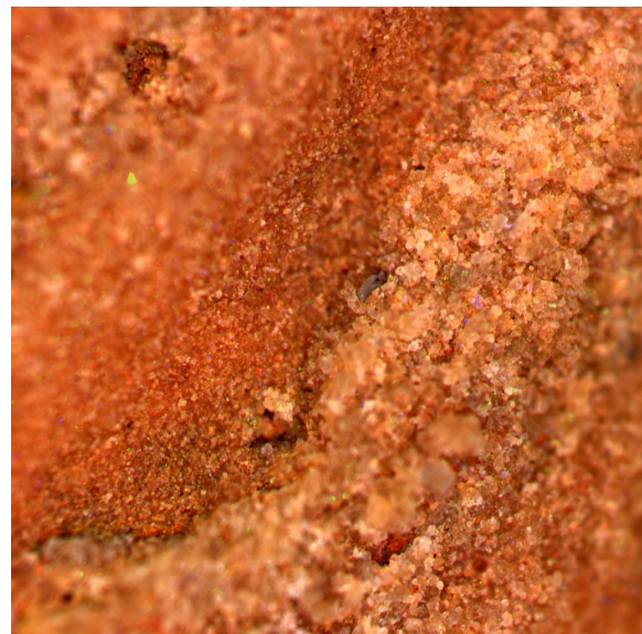
Fig. 58: An image of a sample of sedimentary rock from Piz Alv in Switzerland taken with the Beagle 2 microscope. MPAE has a collaboration with the Natural History Museum in Bern, Switzerland (B. Hofmann) to investigate Mars analogues with the microscope.
