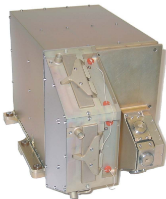
Fig. 46: View of the RAPID instrument (Research with Adaptive Particle Imaging Detectors)
