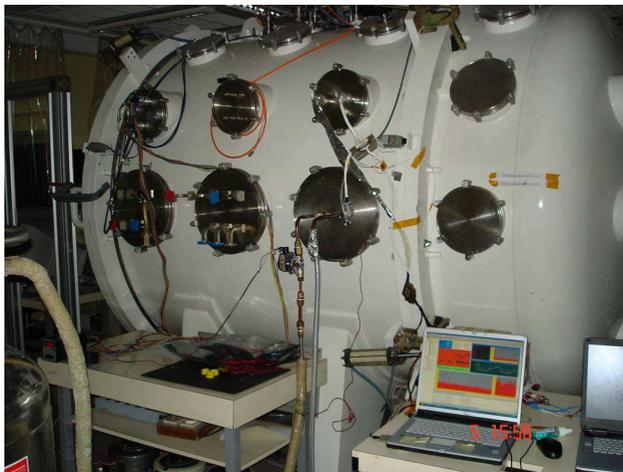
Figure 4.1: The 1.7 meter thermal vacuum chamber at ISRO. The window of the chamber is on the left (not shown).
