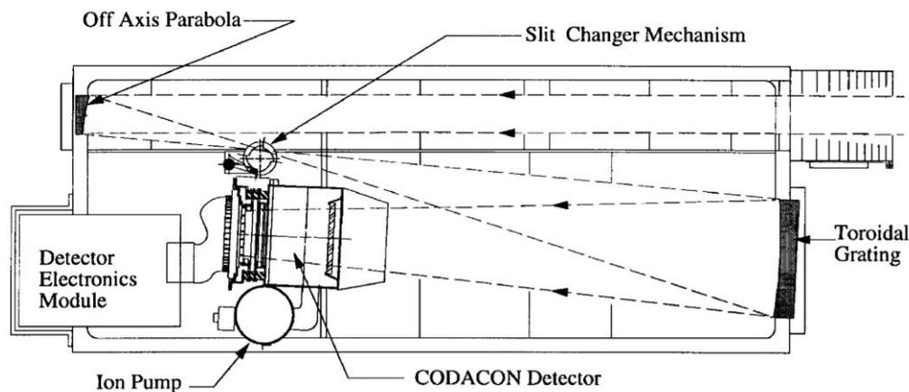
Figure 2.7: Optical design of the UVIS FUV telescope-spectrograph. From Esposito et al. (2004).
