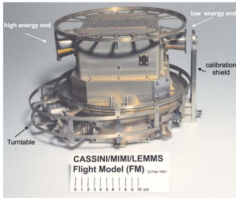
Figure 2.4: Flight model of the MIMI/LEMMS sensor. The double heads of the detector head surrounds the central electronic box which is mounted on the turntable platform, while the calibration shield is used to perform background measurements. From Krimigis et al. (2004).
