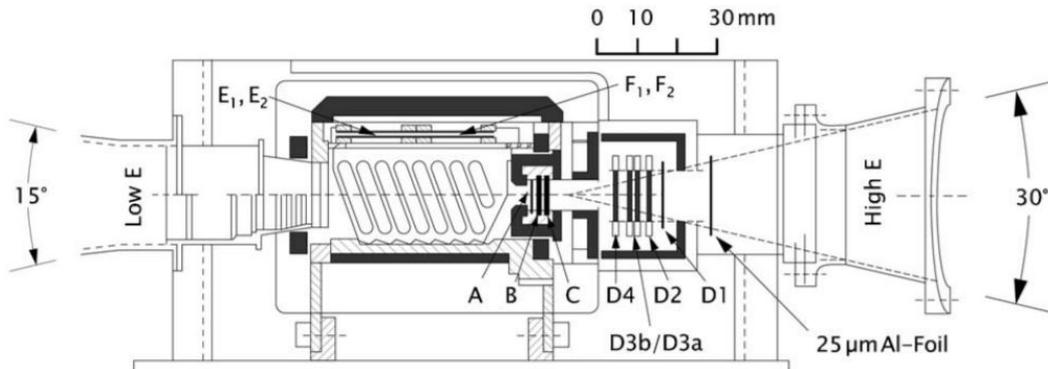
Figure 2.6: Side view of the MIMI/LEMMS double-ended detector, with the Low-Energy Telescope on the left and the High-Energy Telescope on the right. From Armstrong et al. (2009).
