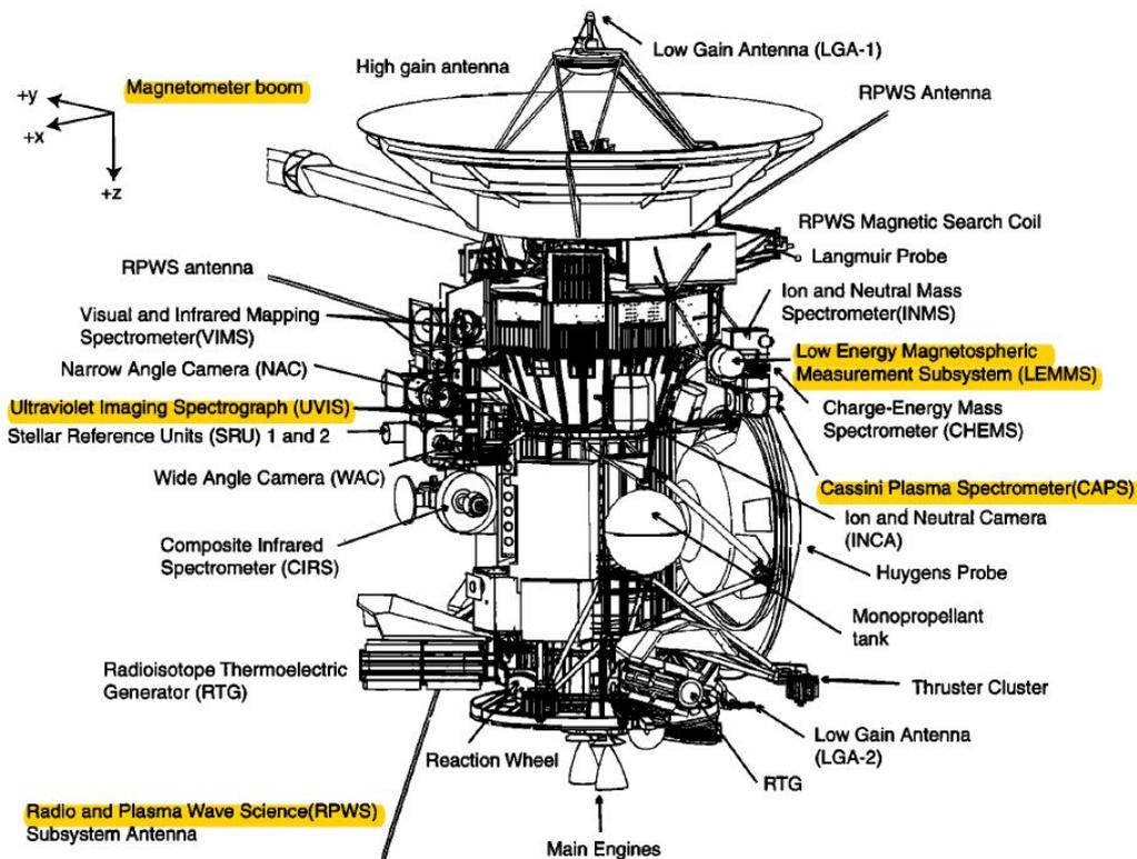
Figure 2.3: Sketch of the Cassini spacecraft with the instruments on board as well as the Huygens probe. The instruments or the sensors whose data have been used in the multi-instrument study presented in this thesis are highlighted. From Burton et al. (2001).
