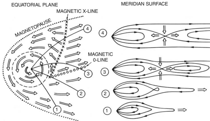
Figure 1.11: Schematic showing the mass loading and release process which are part of the Vasyliūnas cycle. The equatorial plane is shown on the left and meridional cuts (with the Sun to the left in both views) on the right. The magnetic X-line and O-line are drawn. Illustration from Bagenal (2013), adapted from Vasyliūnas (1983).
