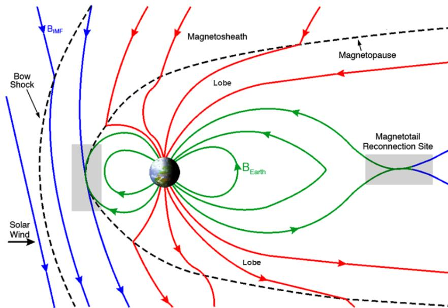
Figure 1.10: Sketch of the Dungey cycle on a noon-midnight meridian plane at the Earth's magnetosphere. From Fuselier and Lewis (2011), adapted from Hugues (1995).
