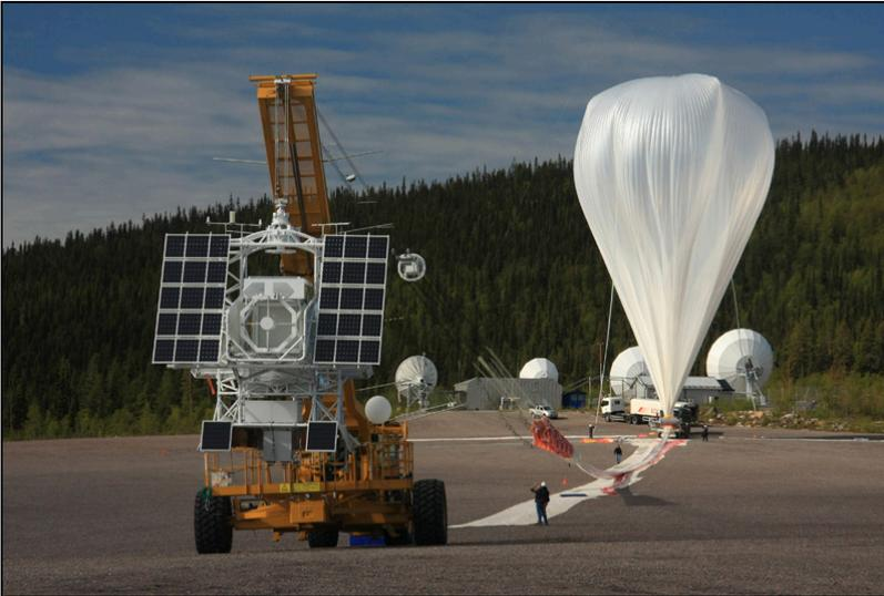
Figure 2.1: SUNRISE balloon-borne solar observatory before launch in Kiruna (northern Sweden). From Barthol et al. (2011).
