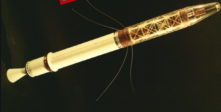
Explorer 1 (Jan 31, 1958) carried a Geiger Counter to study the latitudinal distribution of low-energy cosmic rays. It failed miserably in that
