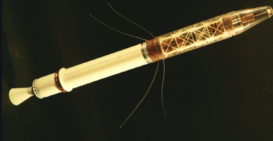
Explorer 1 (Jan 31, 1958) carried a Geiger Counter to study the latitudinal distribution of low-energy cosmic rays. It failed miserably in that
