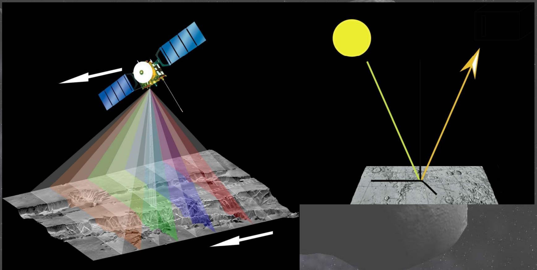
Operation principle of a scanning camera (HRSC / Mars Express).
