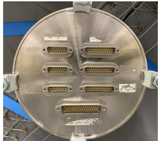
Figure 10.6: A DN160 Electrical flange with Sub-D connectors
