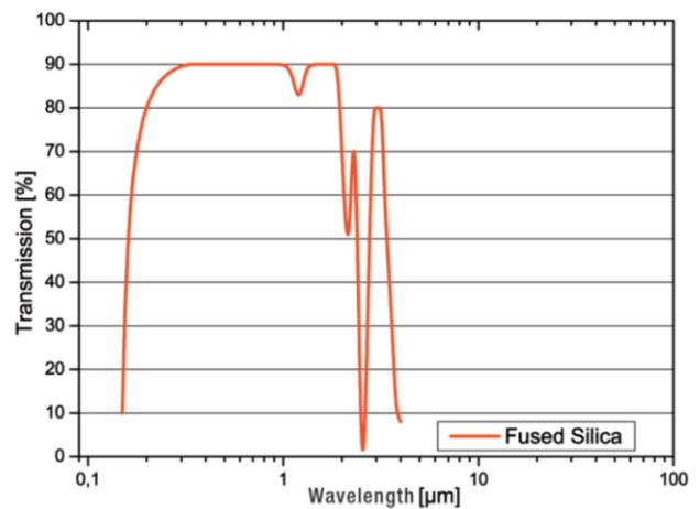
Figure 10.8: Optical Glass, Fused Silica (Synthetic Amorphous Quartz)
