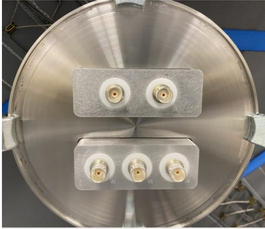
Figure 10.3: Flange DN160 with Coax-Press connectors
