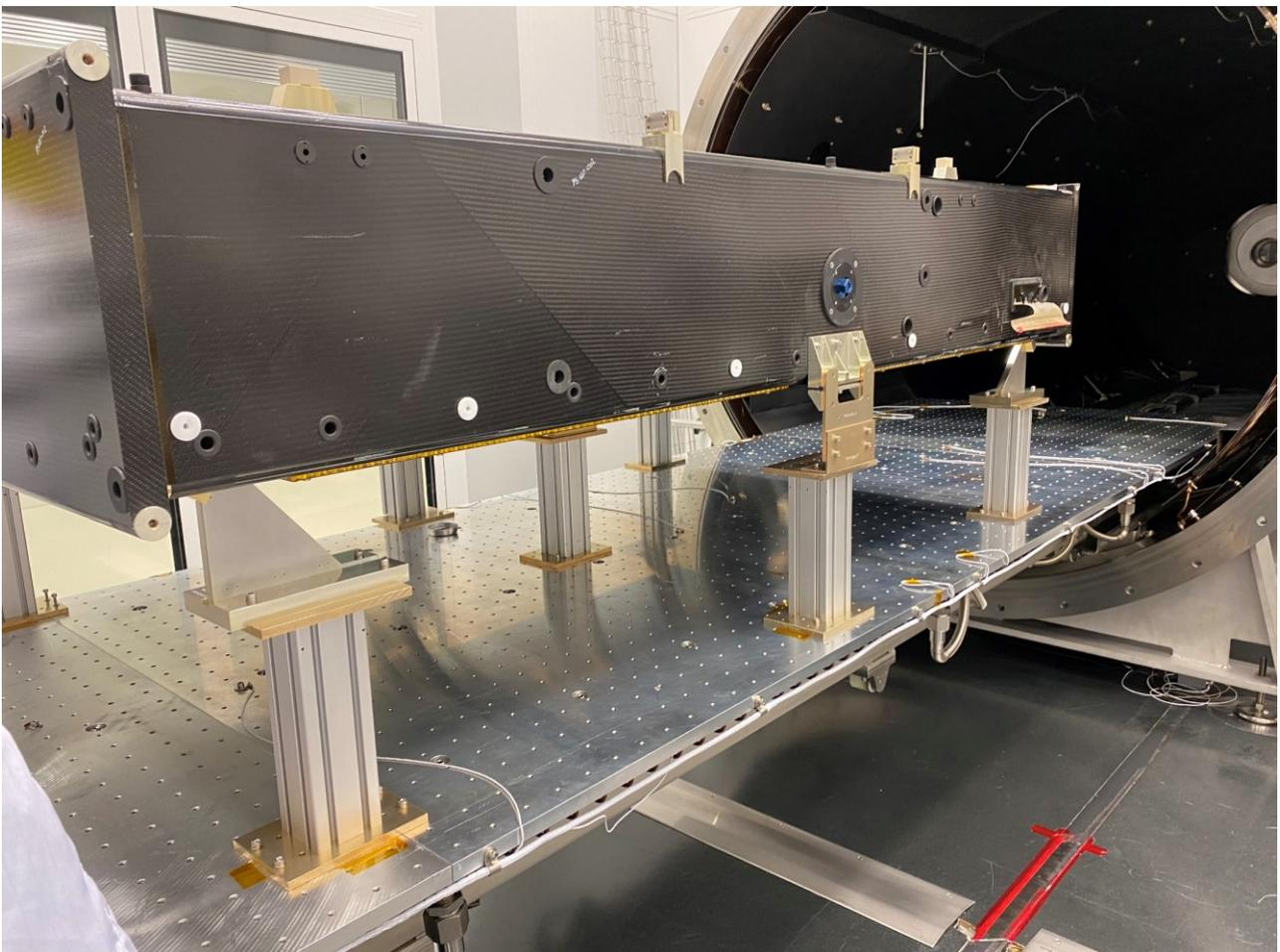
Figure 10.1: Adapters to raise the PFI to be in line with Bigmac optical axis.
