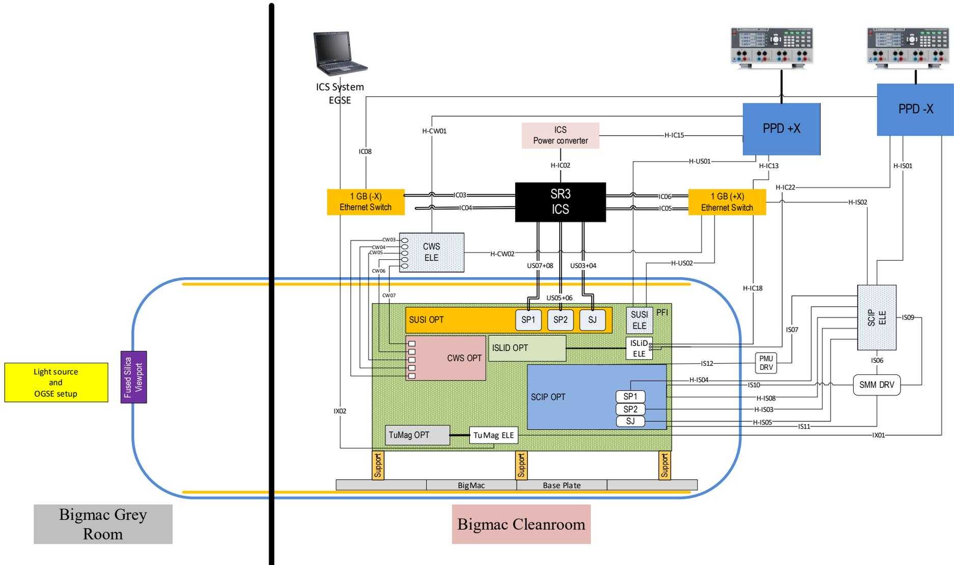
Figure 9.2: Electrical schematics for PFI Vacuum Test – updated.
