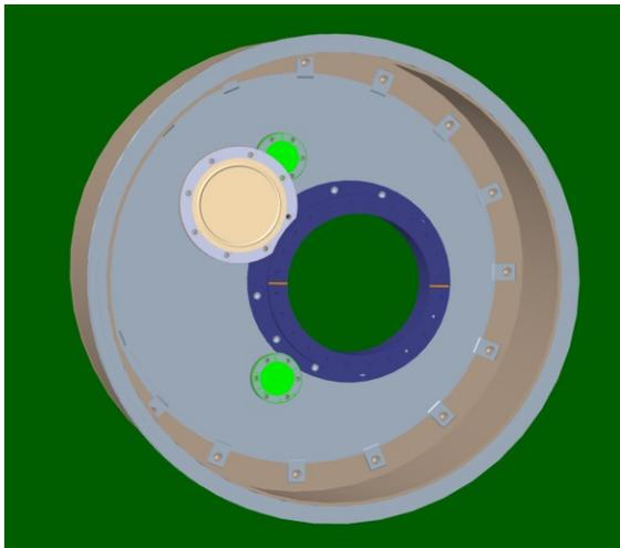
Figure 10.7: DN200 Fused Silica on DN300 KF flange.
