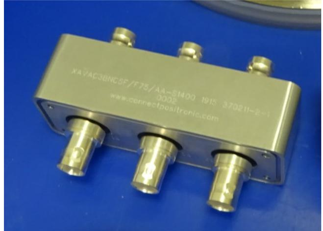
Figure 10.4: CoaxPress BNC 75Ω connectors
