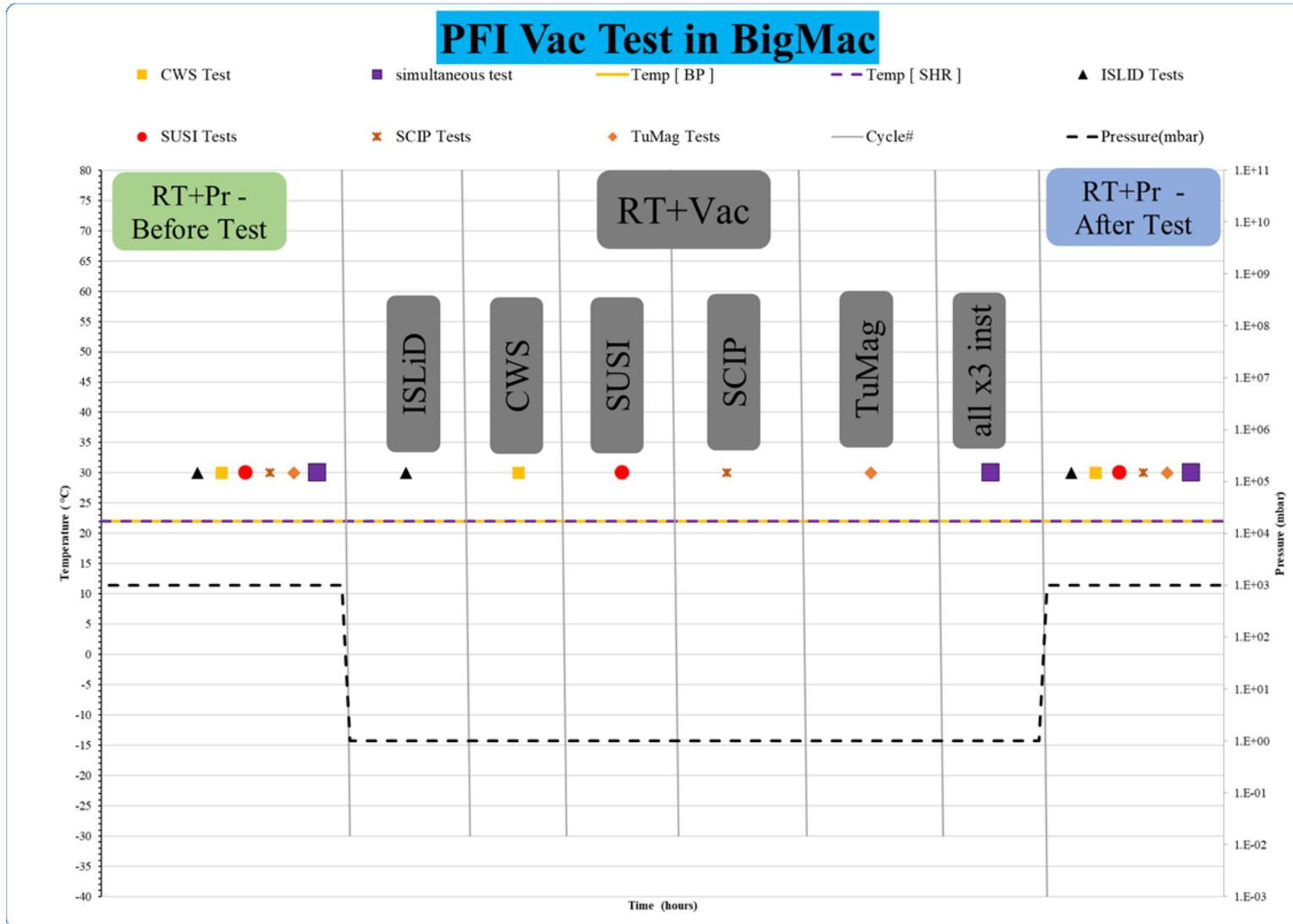
Figure 9.1: PFI Vacuum test sequence
