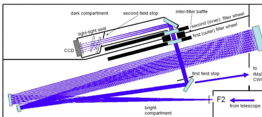
Figure 1.11: Optical layout of SUFI. The layout is optimized for low parasitic light. The two plates in front of the CCD show the phase diversity plates described in Sect. 1.3. Taken from [Gandorfer et al. \(2011\)](#).
