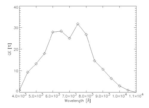
Figure 3.2: LASCO C3 CCD detector quantum efficiency (Cook 1994).
