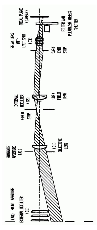
Figure 3.1: Optical scheme of the LASCO C3 coronagraph.
