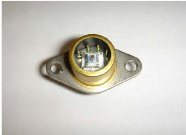
Fig. 7 Single photon detector, quantum efficiency \rho = 0.4 at 532 nm, diameter = 40 \mu\text{m}
