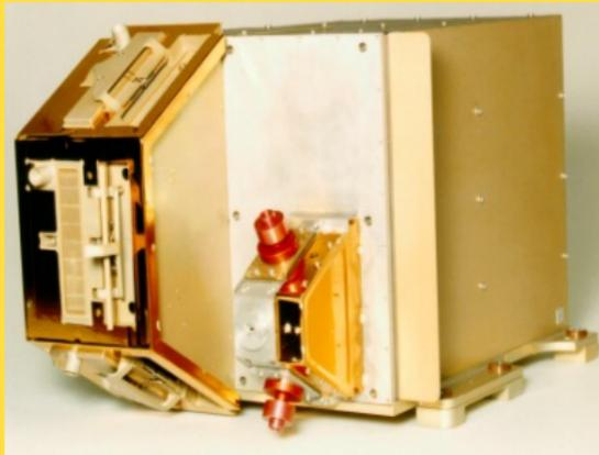
is the energetic particle spectrometer on board Cluster is an advanced particle detector for the analysis of suprathermal plasma distributions in the energy range from 20–400 keV for electrons, 40 keV–1500 keV for hydrogen, and 10 keV/nucleon–1500 keV for heavier ions.
